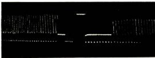
Fig. 9. Video output to illustrate use of a zero carrier reference pulse.
