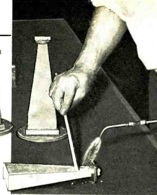
Fig. 3. Joining metal pieces to form a tapered wave guide adapter.
